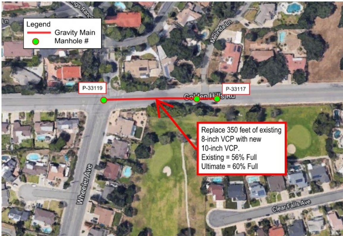
Figure 6.2 – Golden Hills Road Pipeline Improvements
